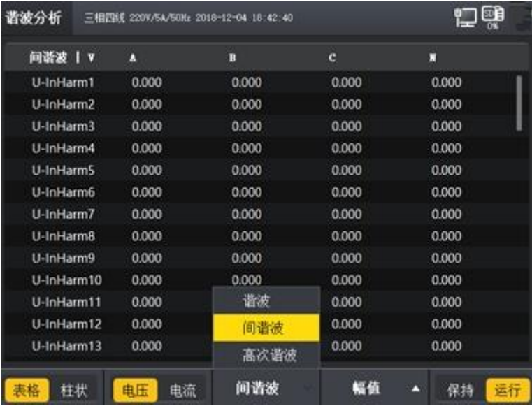
Figure8-9Harmonic Analysis - Harmonic Switching
